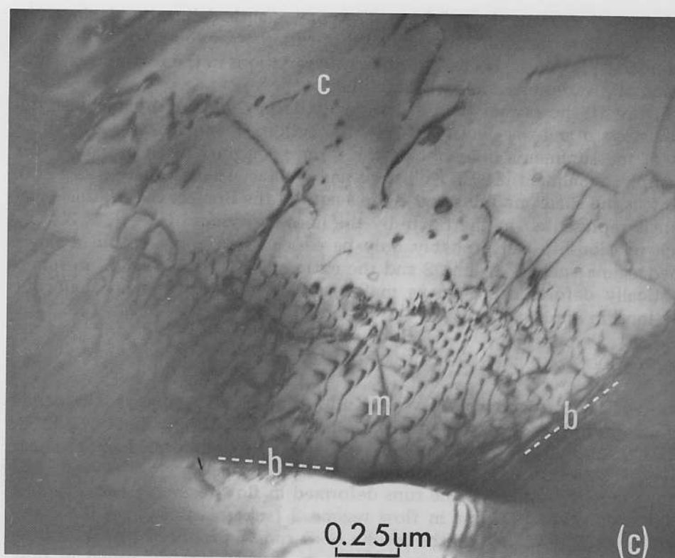
Fig. 11. Transmission-electron microscopy of the dislocation substructures. (a) Test 2550 deformed in regime 2, 12% shortening ( 600^{\circ} , 10^{-5} sec ^{-1} ). (b) Test 2569 deformed in regime 3, 36% shortening ( 900^{\circ} , 6.7 \cdot 10^{-4} sec ^{-1} ). (c) Test 2554 deformed in regime 3, 28% shortening ( 800^{\circ} , 10^{-5} sec ^{-1} ); c = core region; m = mantle region; b = grain boundaries.
