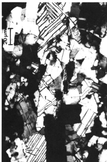
Fig. 4. Optical micrograph of specimen AWP 98 deformed at 450^{\circ}\text{C} , 4.5 \times 10^{-5} \text{ sec}^{-1} , 50% shortening. The micrograph is taken in the vicinity of the piston, where the strain is locally very small. Note that only small portions of a grain are in a twinned orientation (marked t ). The compression axis is N–S in this and all the following micrographs.
